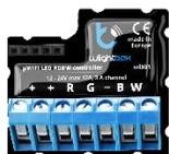
wLightBox is the world's smallest wireless LED light which allows you to control colourful (RGB + W) and mono-colour LED lighting. It is supported not only by smartphones and tablets, but also laptops, personal computers and other modern devices.
