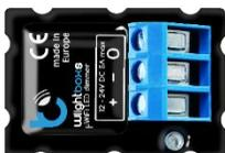
**wLightBoxS** is a miniature device that allows you to control the brightness of single color LED lighting by using smartphones and tablets.
