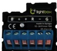
LightBox is the world's smallest, wireless controller based on the Bluetooth technology of the fourth generation. It allows you to control lighting LED lighting - LED color (RGB) and single-color using a smartphone or tablet.
